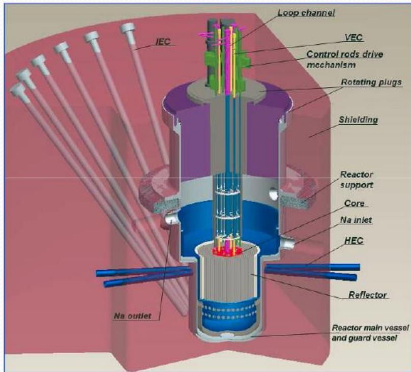
Lay-out of the MBIR reactor vessel and its experimental channels
